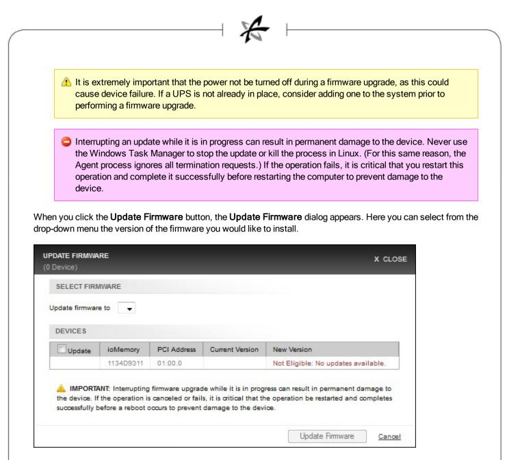
The selected ioMemory device(s) appear below the Update firmware drop-down menu. Check the corresponding checkbox to perofrm the desired action on the selected device or devices.
